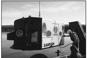
Triton Logging Company's Sawfish Underwater Harvester is a new piece of marine technology. It operates via remote pilot and can operate at any depths. It has a feller grapple and 55-inch chainsaw to cut trees via eight built-in video cameras and sonar. It deploys reusable air bags that attach to the trees to float them to the surface. It may find a use in the Missouri River.
