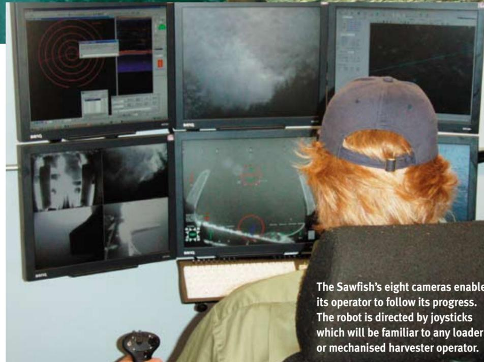
The Sawfish's eight cameras enable its operator to follow its progress. The robot is directed by joysticks which will be familiar to any loader or mechanised harvester operator.
