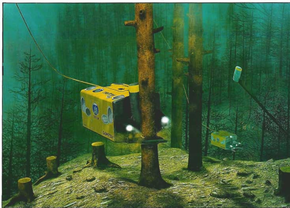
The Sawfish grabs the tree with 4-foot grapples, attaches an airbag, and then cuts the tree - the airbag providing lift to the waterlogged tree.
