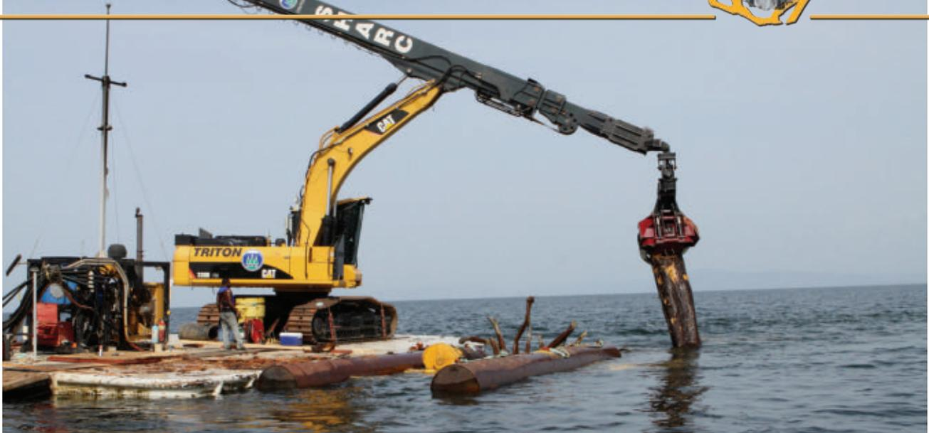
Triton Logging's new Sharc underwater harvester can reach submerged trees in relatively shallow lakes, depositing them in floating bunks for transportation to a mill.
