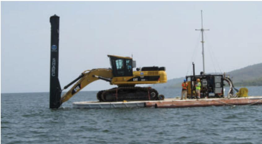
Both barge and boom are powered by a Caterpillar C9 diesel engine. One engine is in the Caterpillar 330D forestry machine, the other in a power unit driving the barge.
